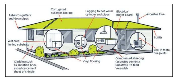
If asbestos is identified during construction, strict procedures must be followed. Work methods, equipment and safety procedures must follow with the New Zealand Guidelines for the Management and Removal of Asbestos and the Health and Safety at Work Act (Asbestos) Regulation 2016.
